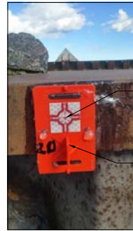
TYPICAL TARGET INSTALLATION
