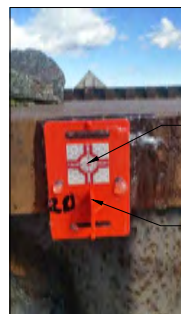
TYPICAL TARGET INSTALLATION
