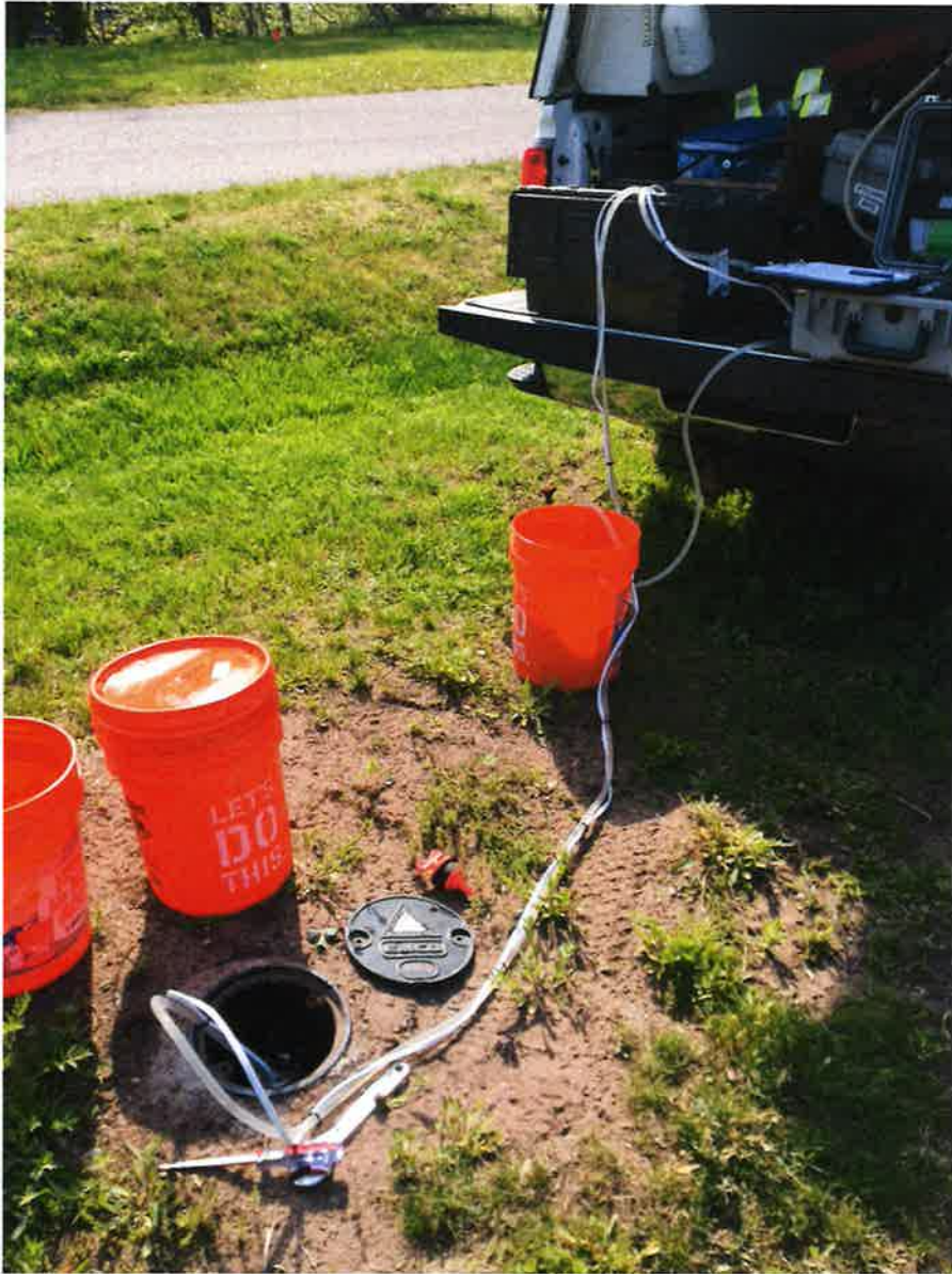
Well development (MW-4)
